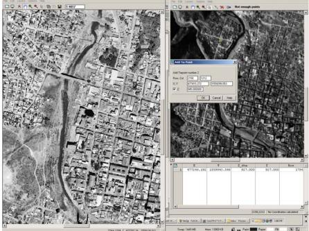
After generating a georeference direct linear with sufficient accuracy, you can then proceed by resampled the airphoto from 1977 to the common georeference used for all the data. This georeference is called "Somewhere".
