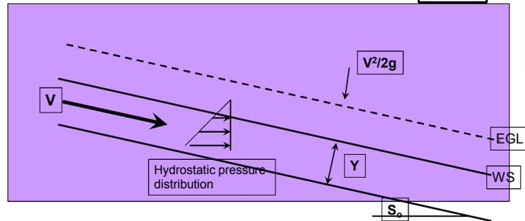
Channel bottom is parallel to water surface is parallel to energy grade line. The streamlines are parallel.
