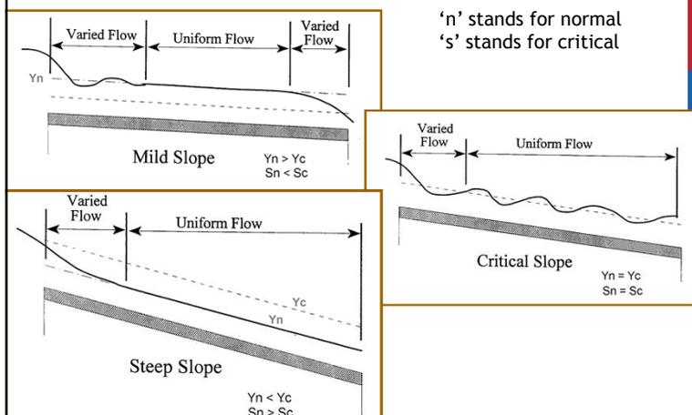
If the flow is a function of the slope and boundary friction, how can we account for it?
