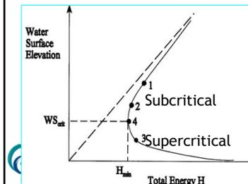
Note: Critical depth is independent of roughness and slope
