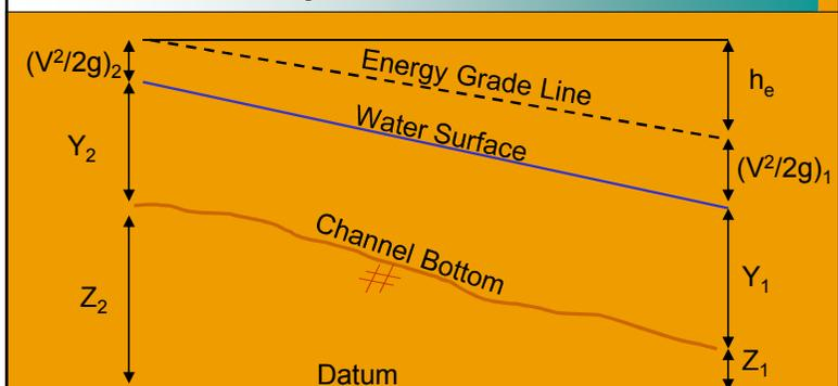
$$WS_2 = WS_1 + \frac{1}{2g} (\alpha_1 V_1^2 - \alpha_2 V_2^2) + h_e$$
